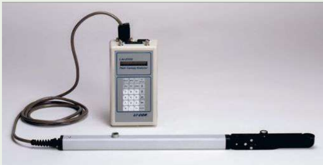
LAI-2000 Plant Canopy Analyzer
